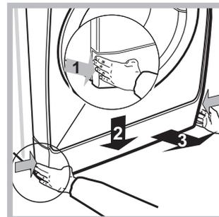
3. remove the cover panel on the lower front part of the washing machine (see *figure*).
